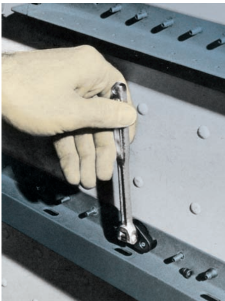
HLH128-8 Tool with HLH130 1/4" Drive Flex Handle is shown removing 1/4" (-8) Hi-Lok collar without damage to pin.
